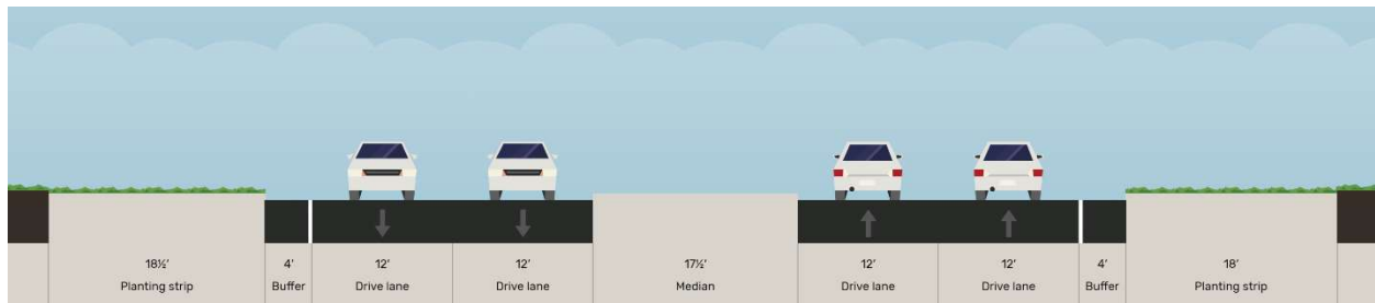
Figure 17: Typical Section 4E – 4 Lane Divided with Paved Shoulders and Sidewalks
